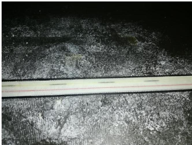
*Figure 2: Inside the 3D printer after the adhesive layer was printed*
